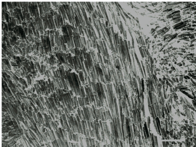
Figure 5. TEM image of an ultrathin slice of tooth enamel. Notice the regional high parallel orientation of the enamel crystals. Scale bar corresponds to 100 nm (Reproduced with friendly permission of the Quintessence Verlag 21 ).
